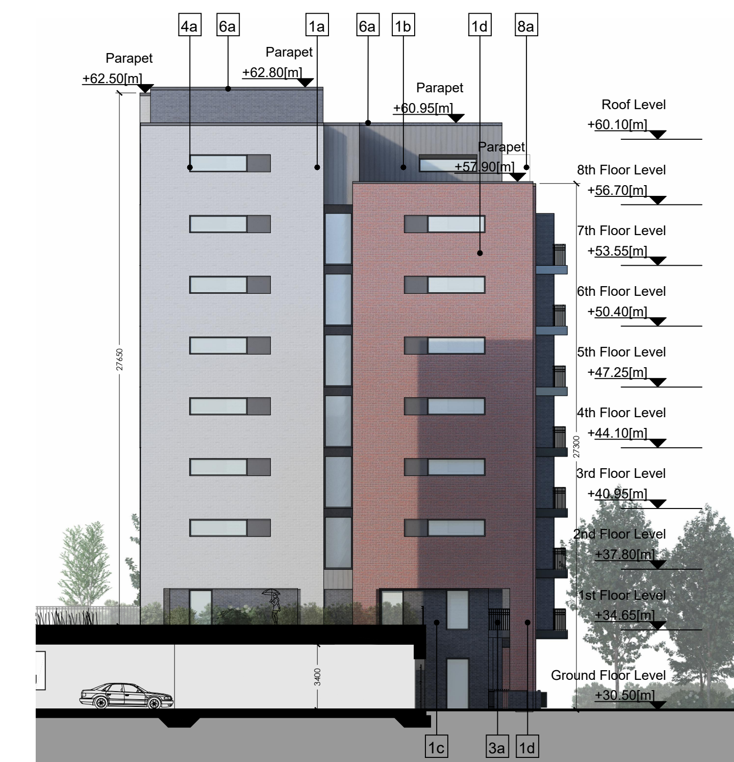
06 - Courtyard North Gable Elevation - Block 1 Scale 1:200 @A0
